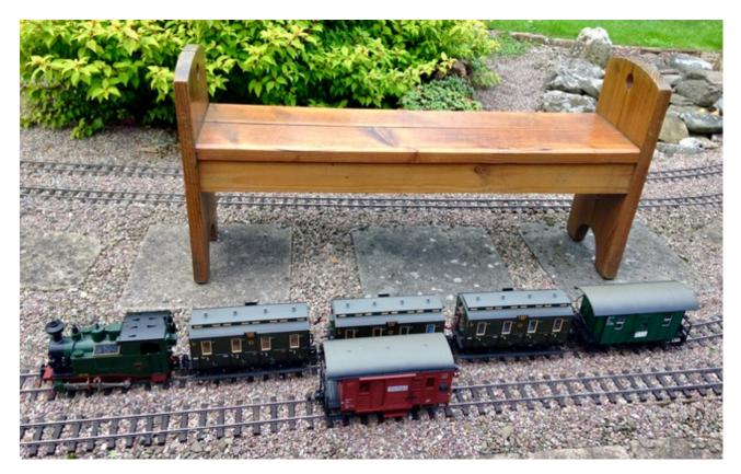
The downside is that there is not a great deal of amps to play with. After a little while say 20 mins. the battery began to run low. The Post van is very heavy to haul as it has two pickup axles with 4 heavy plunger pick ups. If pushed it will not roll along and is about the same number of 'units' as pulling one large bogie coach. (The W&L consider their large bogie coaches to be one and a half units)
